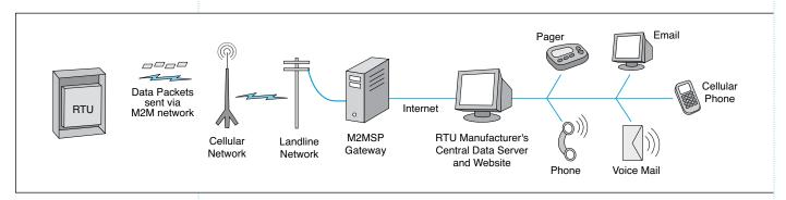
The RTU gathers information that is sent in "data packets" from the transceiver via the M2M portion of the cellular network, and on to the region's cellular tower. Then, the data packets are transmitted via the landline network to the M2M service provider
