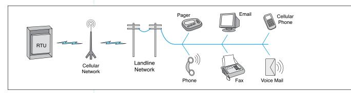
The RTU uses a cellular fixed wireless terminal (CFWT), rather than a landline, to send information. The RTU obtains information from the unattended
