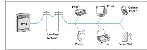
The RTU obtains information from the unattended equipment and sends it via the landline network to multiple predetermined destinations.
